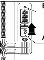
1. Set the combination to the factory default number. To test it, check whether the opener **A** can be pushed up. While setting the new combination leave the zip puller outside the lock.
